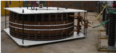
Figure 2: Power transformer model.
